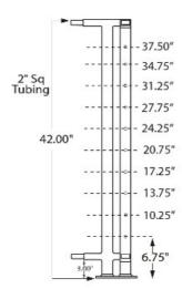
These CS508 prefabricated posts are 2" square posts, 42" high for cable rail and are made of aluminum. They include pre-drilled holes, a welded flange, and necks on the top and the bottom to fit with rectangular tube 2" x 1". Cable kits are available in both 1/8" and 3/16" thickness.
