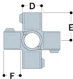
The unique "Hinge and Pin" system of this fitting enables existing structures to be easily extended without the need for dismantling. This fitting is most frequently used in multiple upright structures to tie a center upright with horizontal pipes in four directions. The upright passes through the fitting.
