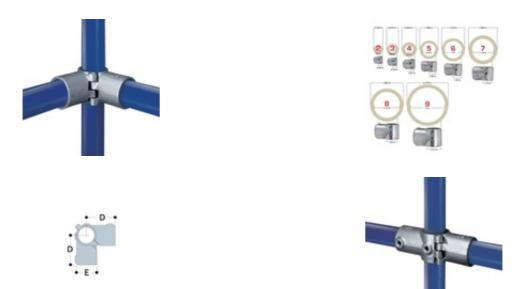
This fitting performs the same function as either KK21 or KK 26, but because of its unique "Hinge and Pin" system, it can be added to an existing tubular assembly. KKA21/A26 fittings are supplied and priced as a kit including 2 castings and 2 taper pins, which can be assembled in either configuration.
