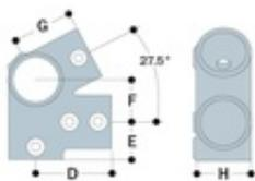
The Type 350 fitting has been designed for small structural building applications and provides for significant load rating. When used with the Type 351 ridge fitting a truss arrangement for additional support can be achieved. Double set screws are provided on the truss outlet to provide additional pull out resistance to hold structures firmly together.
