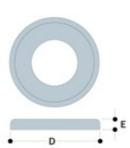
The Cover Flange slips over uprights to finish below ground post installations. The fitting is secured to the upright pipe with a single recessed grub screw.
