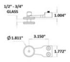
Glass holder designed to hold 1/2 - 3/4 inch thick glass.
