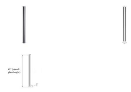
Scenic posts are made of aluminum and are 2-1/2" square in size. These posts are 42" high and have an integral channel designed to hold glass.
