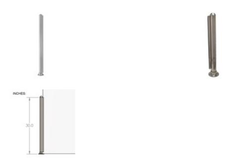
The 44-PR55/E Divider Booth Post is made of brushed (satin) 304 grade stainless steel, 1-1/2" round tube, has a height of 30", and is designed to hold a 1/4" thick panel. Each post comes with a half-ball end cap on top, a round flange attached at the bottom, and one u-channel that holds a panel in place.
