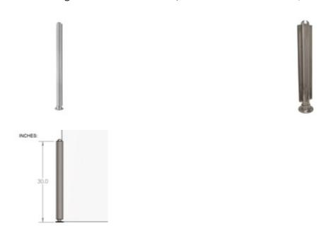
The 44-PR55/C Divider Booth Post is made of brushed (satin) 304 grade stainless steel, 1-1/2" round tube, has a height of 30", and is designed to hold 1/4" thick panels. Each post comes with a half-ball end cap on top, a round flange attached at the bottom, and two u-channels that hold the panels in place.
