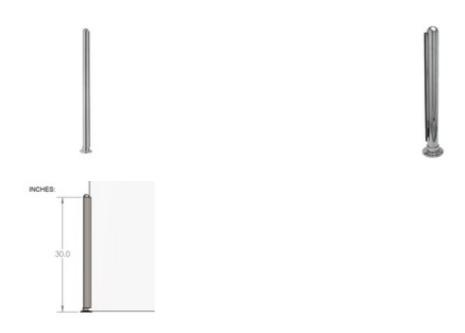
The 40-PR55/E Divider Booth Post is made of polished 304 grade stainless steel, 1-1/2" round tube, has a height of 30", and is designed to hold a ¼" thick panel. Each post comes with a half-ball end cap on top, a round flange attached at the bottom, and one u-channel that holds a panel in place.
