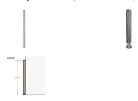
The 40-PR55/C Divider Booth Post is made of polished 304 grade stainless steel, 1-1/2" round tube, has a height of 30", and is designed to hold 1/4" thick panels. Each post comes with a half-ball end cap on top, a round flange attached at the bottom, and two u-channels that hold the panels in place.
