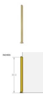
The 00-PR55/E Divider Booth Post is made of brass, 1-1/2" round tube, has a height of 30", and is designed to hold a <sup>1</sup>/4" thick panel. Each post comes with a half-ball end cap on top, a round flange attached at the bottom, and one u-channel that holds a panel in place.
