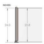
The 44-PR53/E Divider Booth Post is made of brushed (satin) 304 grade stainless steel, 1-1/2" round tube, has a height of 24", and is designed to hold a ¼" thick panel. Each post comes with a half-ball end cap on top, a round flange attached at the bottom, and one u-channel that holds a panel in place.
