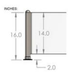
The 44-PR51/E Divider Booth Post is made of brushed (satin) 304 grade stainless steel, 1-1/2" round tube, has a height of 16", and is designed to hold a 1/4" thick panel. Each post comes with a half-ball end cap on top, a round flange attached at the bottom, and one u-channel that holds a panel in place.
