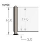
The 44-PR51/C Divider Booth Post is made of brushed (satin) 304 grade stainless steel, 1-1/2" round tube, has a height of 16", and is designed to hold 1/4" thick panels. Each post comes with a half-ball end cap on top, a round flange attached at the bottom, and two u-channels that hold the panels in place.
