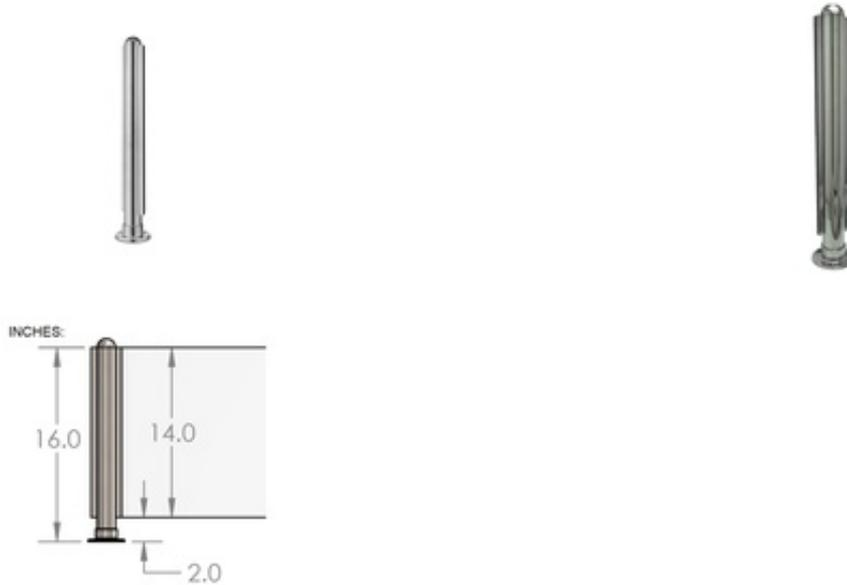
The 40-PR53/C Divider Booth Post is made of polished 304 grade stainless steel, 1-1/2" round tube, has a height of 20", and is designed to hold 1/4" thick panels. Each post comes with a half-ball end cap on top, a round flange attached at the bottom, and two u-channels that hold the panels in place.
