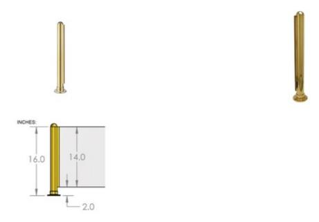
The 00-PR51/E Divider Booth Post is made of brass, 1-1/2" round tube, has a height of 16", and is designed to hold a 1/4" thick panel. Each post comes with a half-ball end cap on top, a round flange attached at the bottom, and one u-channel that holds a panel in place.
