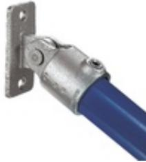
A swivel fitting for attachment of angled pipe to a flat surface. For dimensions refer to KKF50 and KKM58. It is not recommended for use as a base flange to support guardrailing, balustrading or other types of structure.
