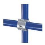
The unique "Hinge and Pin" system of this fittings enables existing structures to be easily extended without the need for dismantling. This fitting is designed to give a 90° offset crossover joint. Pipe should not be joined within the fitting. KKA45 function is comparable to KK45 fittings.
