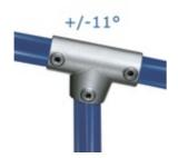
Used to join the top rail to an intermediate upright on a guardrail on a slope from  $0^{\circ}$  to  $11^{\circ}$ . As there are two socket set screws in the sleeve, this fitting can be used to join two ends of rail.
