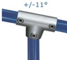
Used to join the top rail to an intermediate upright on a guardrail on a slope from 0° to 11°. As there are two socket set screws in the sleeve, this fitting can be used to join two ends of rail.
