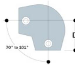
Used to join the top rail to an end upright on a guardrail on a slope from 0° to 11° at both top and bottom of the run.
