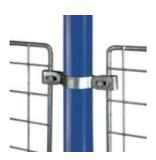
Double clips for attaching wire-mesh infilling. For economy it is possible to use Type 82 clips without the safety attachment, to secure various types of infill panels (plyboard, perspex, etc.) up to a thickness of 25/64". All clips are supplied with hexagonal head fixing bolts, M6x35mm long, and nut. Ø indicates diameter of the safety attachment bolt hole. The primary clip has a slot measuring 8mm x 15mm.
