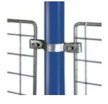
Double clips for attaching wire-mesh infilling. For economy it is possible to use Type 82 clips without the safety attachment, to secure various types of infill panels (plyboard, perspex, etc.) up to a thickness of 25/64". All clips are supplied with hexagonal head fixing bolts, M6x35mm long, and nut. Ø indicates diameter of the safety attachment bolt hole. The primary clip has a slot measuring 8mm x 15mm.
