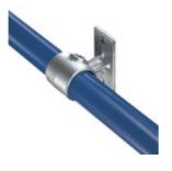
This fitting, with holes provided for countersunk flat head screw fixings only, is designed to carry handrails along walls or to fix structures back to walls. The pipe passes through the fitting and cannot be joined within the fitting. KK70 is also used to attach toeboards to the base of guardrail uprights. Ø indicates diameter of fixing holes. These fittings are not to be used as base flanges for full height guardrails.
