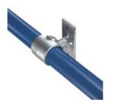
This fitting, with holes provided for countersunk flat head screw fixings only, is designed to carry handrails along walls or to fix structures back to walls. The pipe passes through the fitting and cannot be joined within the fitting. KK70 is also used to attach toeboards to the base of guardrail uprights. Ø indicates diameter of fixing holes. These fittings are not to be used as base flanges for full height guardrails.
