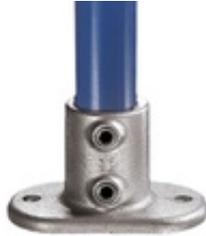
Ideal when a structural fixing is required. When fixing guard railing and balustrades, Type 62 should always be used. The holes are of sufficient diameter to insure proper fixing with either a mechanical or chemical anchor. The two set screws in the vertical socket give greater sideload stability to the upright. It is recommended that the fixing holes in the flange should be in line with the applied load. Ø indicates diameter of fixing holes.
