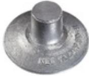
A spigot flange which fits inside the pipe and is not secured by a set screw. Type 59 can only be used with pipe wall thickness of 1/8" and in light, self supporting structures. Type 59 is manufactured in aluminum. No fixing holes are provided in this fitting.
