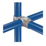
Used on racking to join horizontal carrying rails to the upright, leaving the socket to take a horizontal tie across the section. For shelved racking it is usual to have the horizontal pipe outside the upright. On pallet racking it is preferable to have the carrying rails inside the upright.
