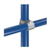
Designed to give a 90° offset crossover joint. Frequently used on safety railing, where, to reduce cost by minimizing the pipe cuts, a continuous horizontal rail is used. Pipe cannot be joined within this fitting. It may be also used to give intermediate levels on racks, etc, when horizontal ties between uprights across the section are not required.
