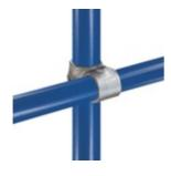
Designed to give a 90° offset crossover joint. Frequently used on safety railing, where, to reduce cost by minimizing the pipe cuts, a continuous horizontal rail is used. Pipe cannot be joined within this fitting. It may be also used to give intermediate levels on racks, etc, when horizontal ties between uprights across the section are not required.
