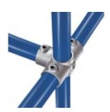
Most frequently used to tie uprights with horizontal pipes in three directions, all at 90° to the upright. The upright passes through the fitting.
