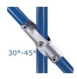
Designed as an alternative to the KK28 fitting, this adjustable fitting can be used for railing on staircases between the midrail and an intermediate upright which is required to remain vertical. It may be used at any selected angle between 30° and 45°.
