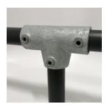
Most commonly used as the 90° joint between the top rail and an intermediate upright on safety railing. As there are two socket set screws in the sleeve, this fitting can be used where a join is required in the horizontal pipe. The KK10 fitting can be used as an alternative when a join in the pipe is not required.
