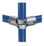
Used in pairs to form variable angle joints between 90° and 180°. When calculating cutting lengths for pipe, dimension 'E' should be subtracted to give true pipe length. In the case of KK19-8 and KK19-85, you can produce an angle range between 60° and 180°. KK19 fittings are normally used in pairs. In the United Kingdom, France, and Germany, they are sold and priced separately. In the USA and Canada, they are sold and priced in pairs.
