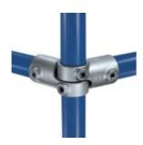
Used in pairs to form variable angle joints between 90° and 180°. When calculating cutting lengths for pipe, dimension 'E' should be subtracted to give true pipe length. In the case of KK19-8 and KK19-85, you can produce an angle range between 60° and 180°. KK19 fittings are normally used in pairs. In the United Kingdom, France, and Germany, they are sold and priced separately. In the USA and Canada, they are sold and priced in pairs.
