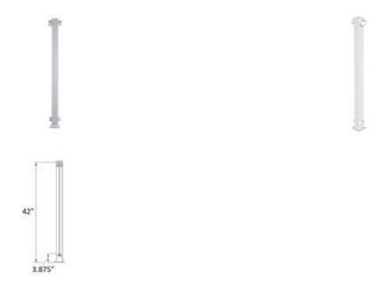
The 42" High Floor Mount Post for glass panels is a 2-1/2" square aluminum post available in center, corner, end and stair configurations. All posts are available in textured black, white and textured lakeside copper premium powder coated finishes.
