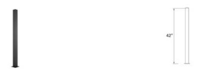
The 42" High Floor Mount Post for glass panels is a 2-1/2" square aluminum post available in center, corner, end and stair configurations. All posts are available in textured black, white and textured lakeside copper premium powder coated finishes.
