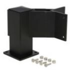
The fascia bracket for 2-1/2" square aluminum posts is made of aluminum and is designed to connect with GS635/36/F and GS635/42/F floor mount posts.
