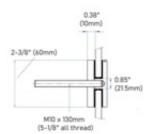
This 2-3/8"round wall mount glass clamp from IAM Desgin is made of 316 grade stainless steel, has a brushed (satin) finish and is designed to hold 5/16 – 21/32" thick glass. It has an offset from the wall to the glass of 0.38" (10mm) and comes complete with a threaded bolt. Mount this bracket on a wall (recommended on a stud) or on a rectangular vertical post using the included hardware or alternate depending on the material the bracket is being mounted upon.
