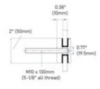
This 2"round wall mount glass clamp from IAM Design is made of 316 grade stainless steel, has a brushed (satin) finish and is designed to hold 5/16 - 21/32" thick glass. It has an offset from the wall to the glass of 0.38" (10mm) and comes complete with a threaded bolt. Mount this bracket on a wall (recommended on a stud) or on a rectangular vertical post using the included hardware or alternate depending on the material the bracket is being mounted upon.
