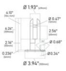
This floor mount round glass clamp from IAM Design is made of 316 grade stainless steel, has a brushed (satin) finish, is 1.93" (49mm) in diameter, and is designed to hold 1/2 and 11/16" thick glass. The flange on the bottom is 3.94" in diameter and has three countersunk holes for mounting to the floor.
