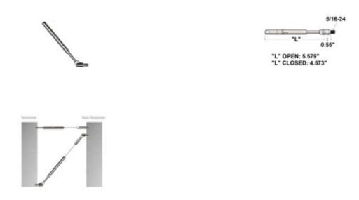
CA-MST1/8-1 is a tensioning cable fitting for stair railing that is designed to mount onto a metal post. This fitting has a swivel feature that allows the cable to be set at an angle. It is made of weather resistant 316 grade stainless steel and is designed to hold 1/8" thick cable. This fitting is made in the USA.
