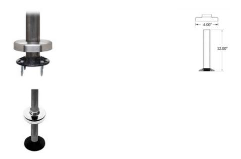
44-B/1H flange, insert, and canopy set is made of a cast iron flange, a steel insert, and a satin (brushed) stainless steel canopy. This set is designed to mate with 1-1/2" OD round tube. The flange has four holes for mounting hardware and a large threaded hole in the middle that mates with the threaded end of the insert.
