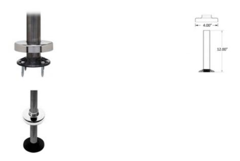
40-B/1H flange, insert, and canopy set is made of a cast iron flange, a steel insert, and a polished stainless steel canopy. This set is designed to mate with 1-1/2" OD round tube. The flange has four holes for mounting hardware and a large threaded hole in the middle that mates with the threaded end of the insert.
