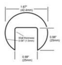
49-A114U architectural round channel tube is available in stainless steel, has a 1.67" outside diameter, a 0.06" wall thickness, and is available in stock lengths up to 16 feet.
