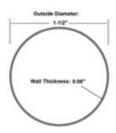
49-A111 architectural round tube is a stainless steel tube with a 1-1/2" outside diameter, a 0.06" wall thickness, and is available in stock lengths up to 20 feet. It is made with 316 grade stainless steel.
