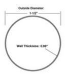
47-A111 architectural round tube is a stainless steel tube with a 1-1/2" outside diameter, a 0.06" wall thickness, and is available in stock lengths up to 20 feet. It is made with 316 grade stainless steel.
