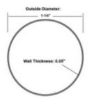
00-A105 architectural round tube is a brass tube with a 1-1/4" outside diameter, a 0.05" wall thickness, and is available in stock lengths up to 12 feet. The alloy is 260. This tube can be used in a variety of applications including, but not limited to
