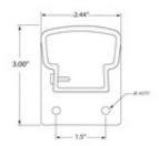
This Top Post End Bracket is made of cast aluminum and is in a white painted finish. It is designed to mount towards the top of our 9000/36/F and 9000/42/F receiver posts and will hold the top rails of our level picket rail panels 3642L.
